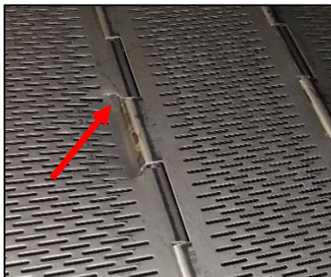
Hinge Knuckle Tear
