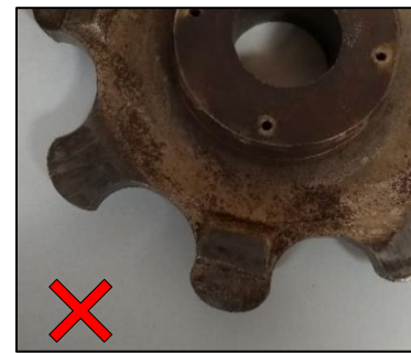
Severely worn sprocket
