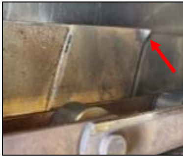
Bent traveling side product guides (TSPGs)
