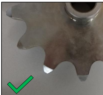
New sprocket (unworn)
